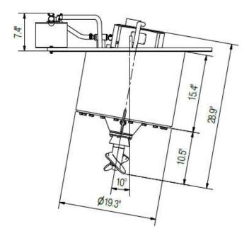
Be aware that the tank must be able to withstand the force from the mixer (both axial and vertical.
